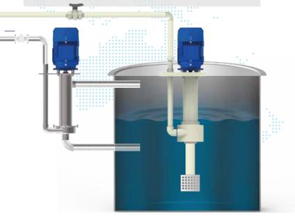
CTV is commonly installed in surface treatment baths, circulating through filter and further to nozzle ramps.
