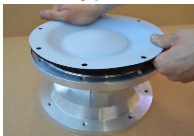
Fig. 3.6.1 Unscrew diaphragm [15] from both sides of the pump.
