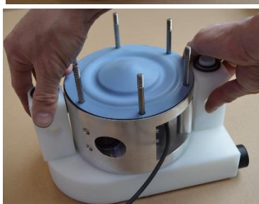
Fig. 3.4.3 Lift the loose manifolds [13] and centerblock [12] from the second housing [11]. Then carefully remove the pin screws [14].
