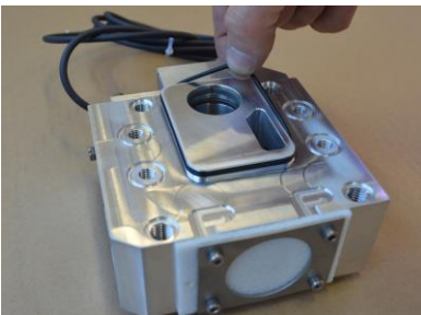
Fig. 3.6.11 Remove back plate square O-ring [1202E] from centerblock groove.
