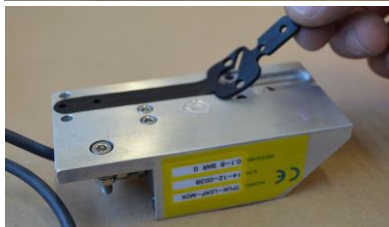
Fig. 3.6.15 Take out the control module [97E]. Take care of the sealing [971E].
