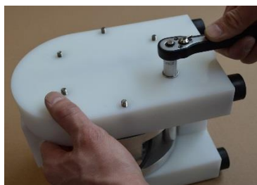
Fig. 3.4.1 Unscrew the housing nuts [37] and washers [38].
