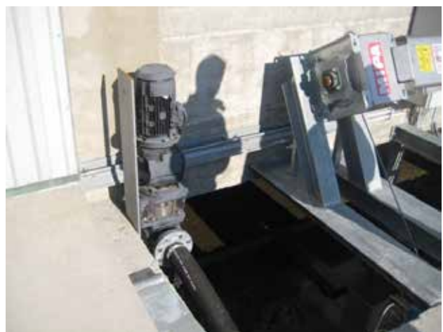
DV pump The machine is immersed directly into the product therefore there is no need for suction pipes which reduces the footprint to the minimum.
