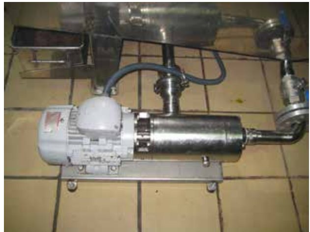
R pump with wobble stator For pumping vegetables waters.
