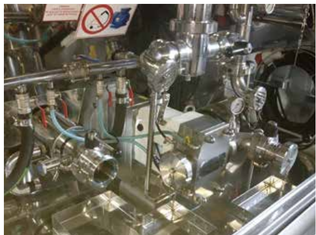
Pumped liquid - transporting syrups, chocolate, etc. Pump - LPX80-1 installed on a truck cistern
