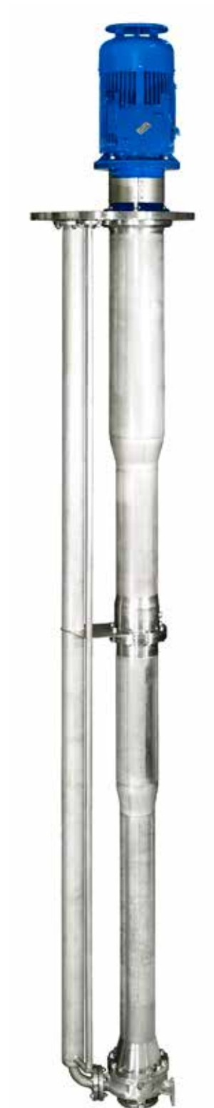
MKTP with motor with jacketed discharge pipe vertical bearing frame mounted (-20 to +175°C)
